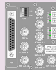
PVD 5840 DO Balanced AES3 Audio 25 pin SubD Connector
