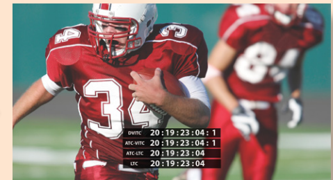
Selectable Timecode Burn In Display up to 4 timecode values Position anywhere on screen
